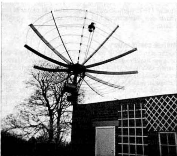
The 23cm dish used for e-m-e work by G3LTF at Chelmsford. Built about two years ago, it uses 1/2" diameter mesh and weighs about 2cwt. The circularly-polarized circular guide feed shown gives good beam concentration: the drop off at the dish edge is -10dB
